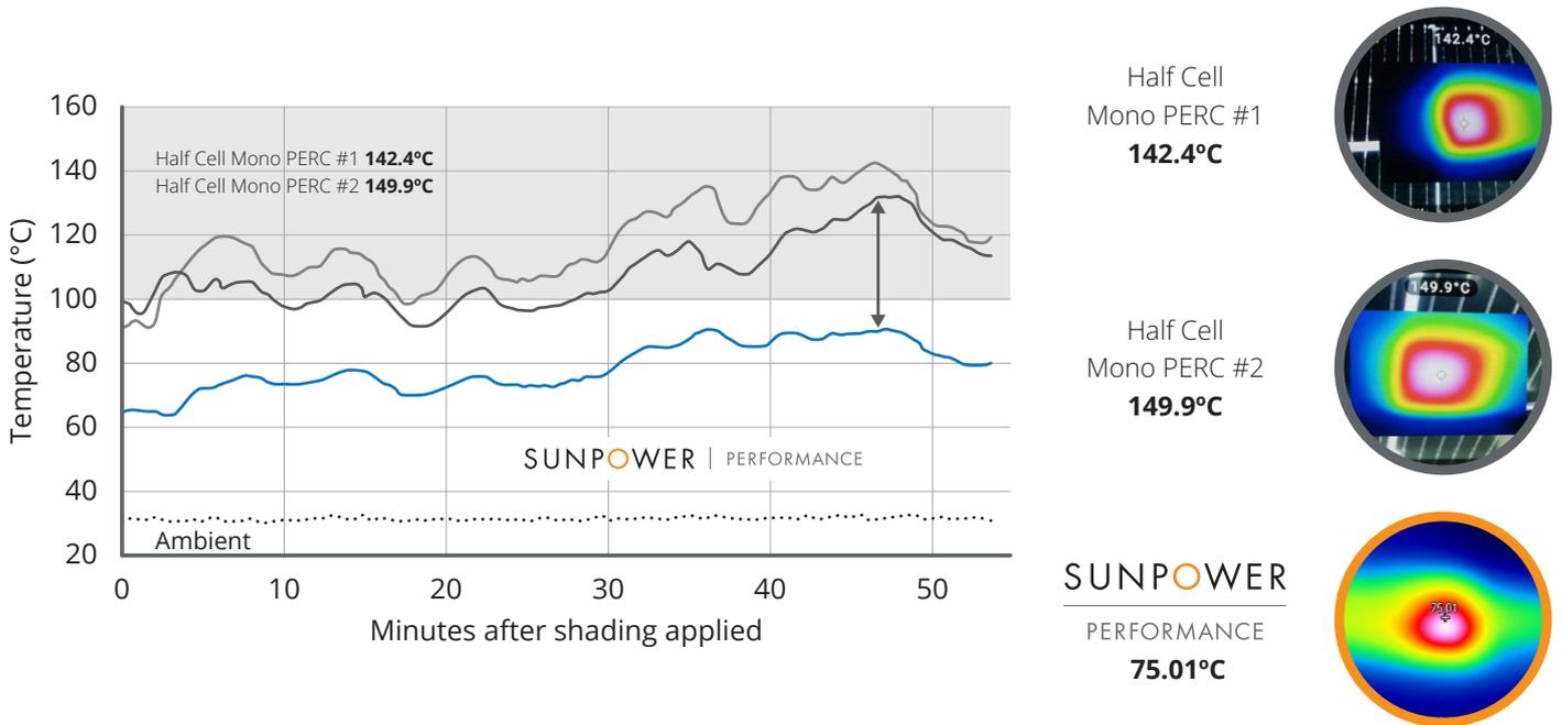
Figure 11: Under severe cell cracking or worst-case shading conditions, Performance panels operate at 40-50°C lower temperature, reducing the risk of temperature-related failures.<sup>9</sup>
