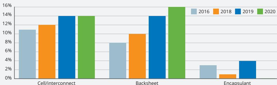
Figure 3: Inspection results from Dupont's Global PV Reliability Field Analysis featuring key causes of panel failure amongst recently installed conventional panels.
